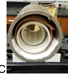
(A) Phantom Samples. (B) Block diagram of homebuilt EFNMR spectrometer. (C) Spectrometer coil assembly. [1]
