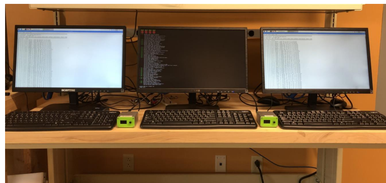
Fig 3. Image of the experimental setup with one central computer, two muon detectors (green), and two signal receiving computers
